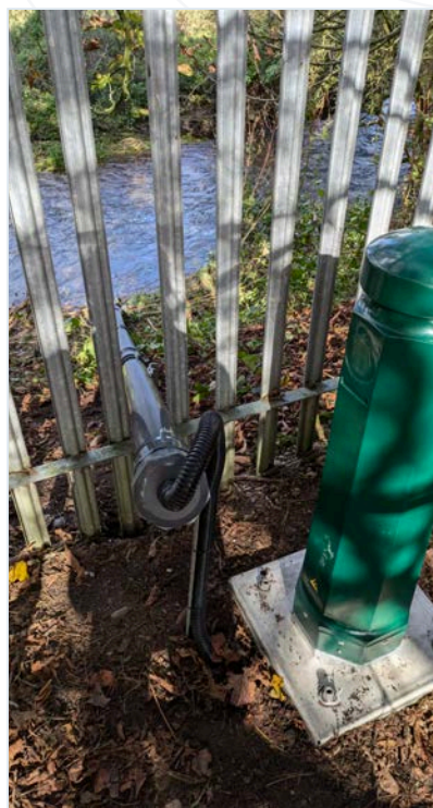
RIVER-LEVEL MONITORING UNIT · UK WATER UTILITY
